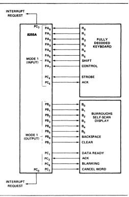
Figure 18. Keyboard and Display Interface
